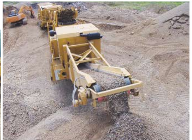
Combination plant featuring a JHT Jaw Crusher & CXT Cone Crusher
