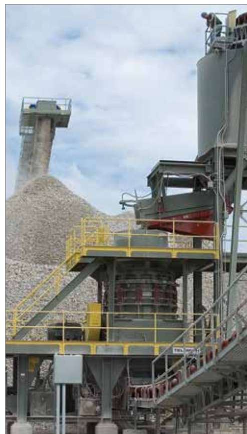
57SBS on a relocate-able modular support structure
