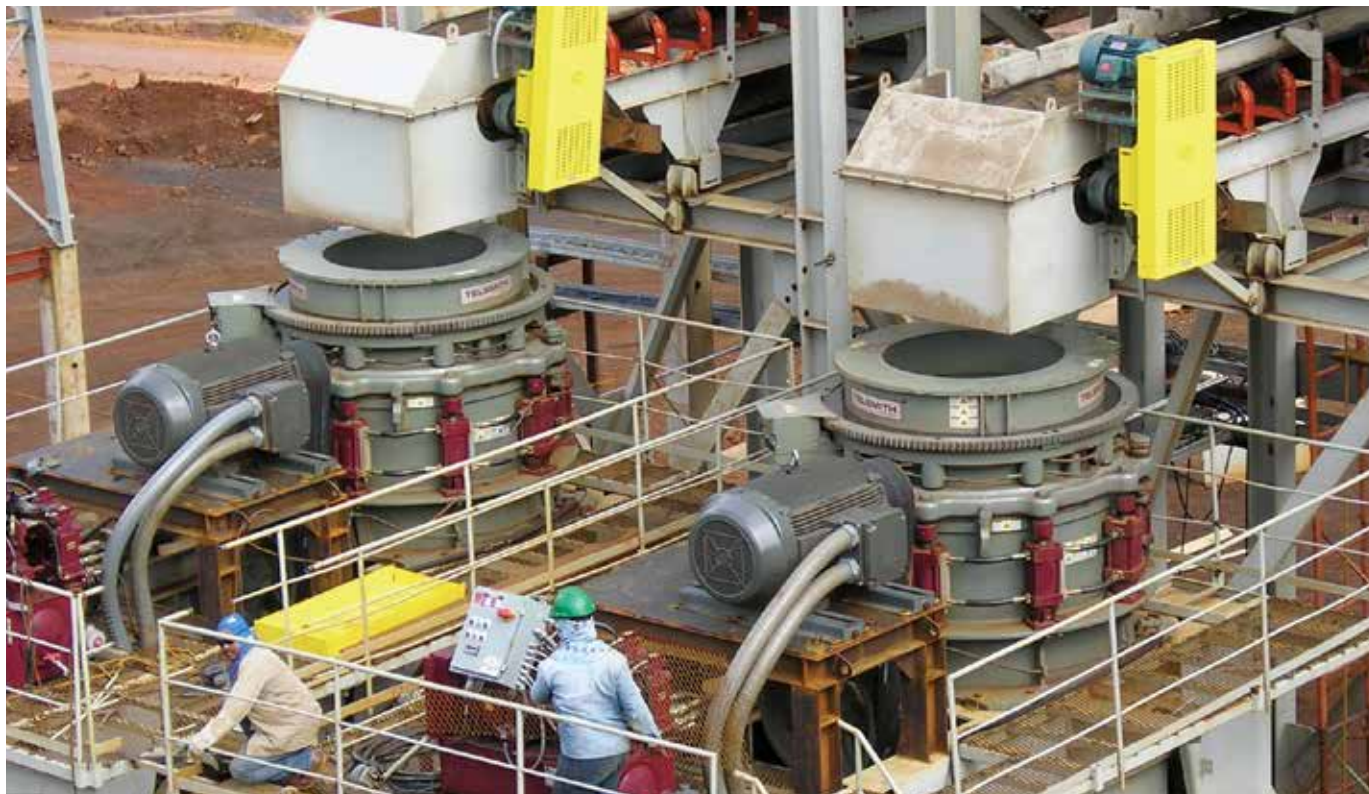
Crushing Iron Ore in Venezuela - two 52SBS cone crushers
