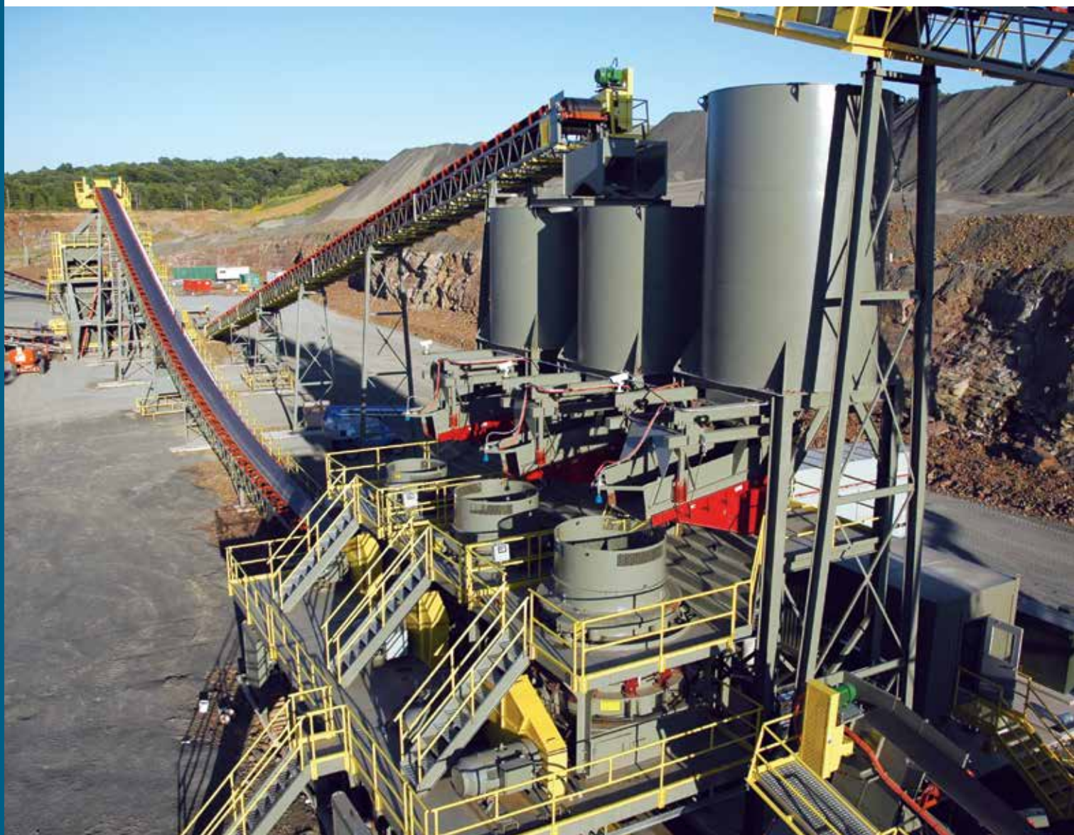
Automated 1000 TPH crushing plant with 68SBS, 57SBS and 52SBS cone crushers
