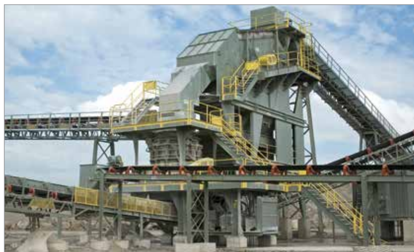
68SBS integrated with 8' x 20' triple deck screen on a modular support structure
